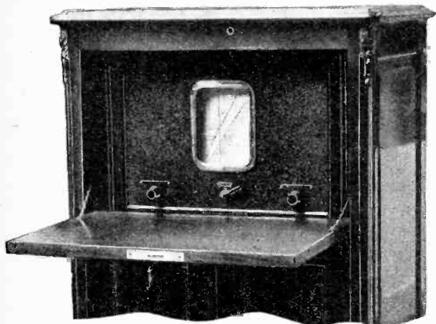
A pair of intersecting cross wires give the tuning positions of the Périscand receiver.
