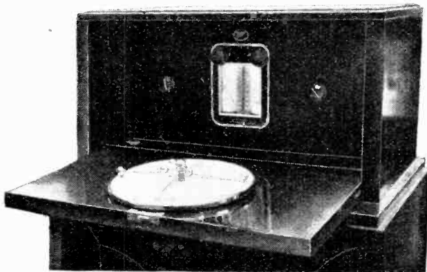
The Berren superheterodyne with calibrated tuning drums and frame-aerial indicator.
