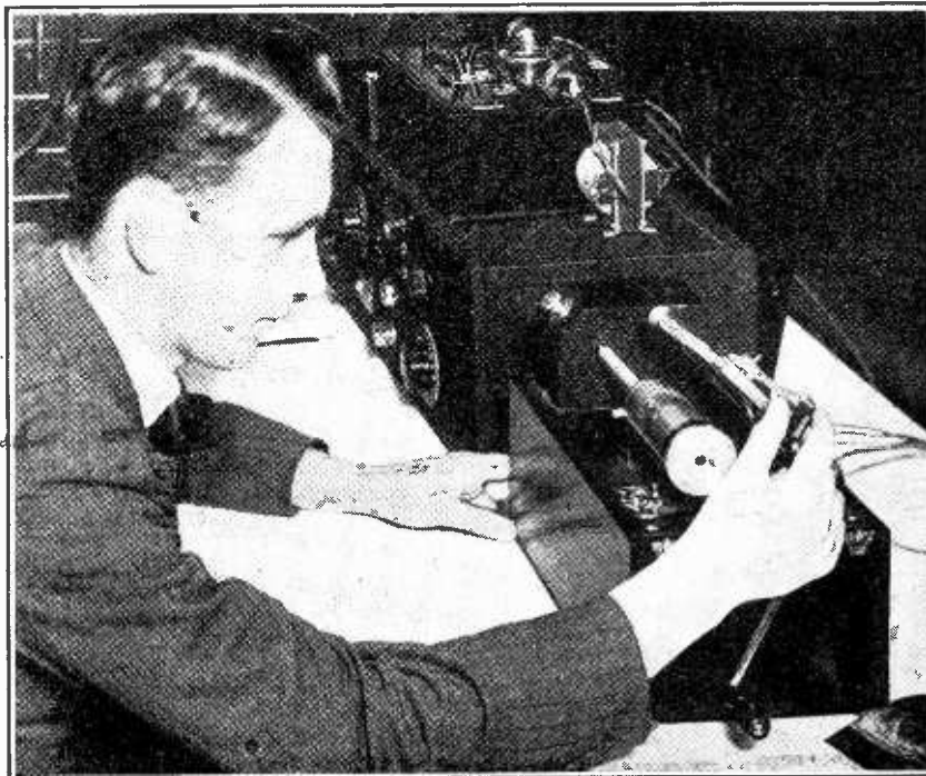
PICTURE BROADCASTING BEGINS. The "Fultograph" transmitting apparatus photographed just before sending the first picture from Daventry, 5XX, on Tuesday, October 30th. The image was transmitted from Savoy Hill by landline to 5XX, whence it was broadcast and picked up on a demonstration set at the Savoy Hotel.
